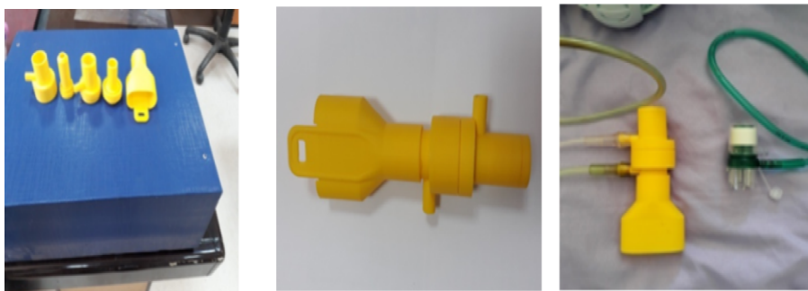
Figure 4: Representation of the CPAP valve that we manufactured (the left image: before assembly, the center image: complete assembly of the valve, the right image: comparison with the original valve).
