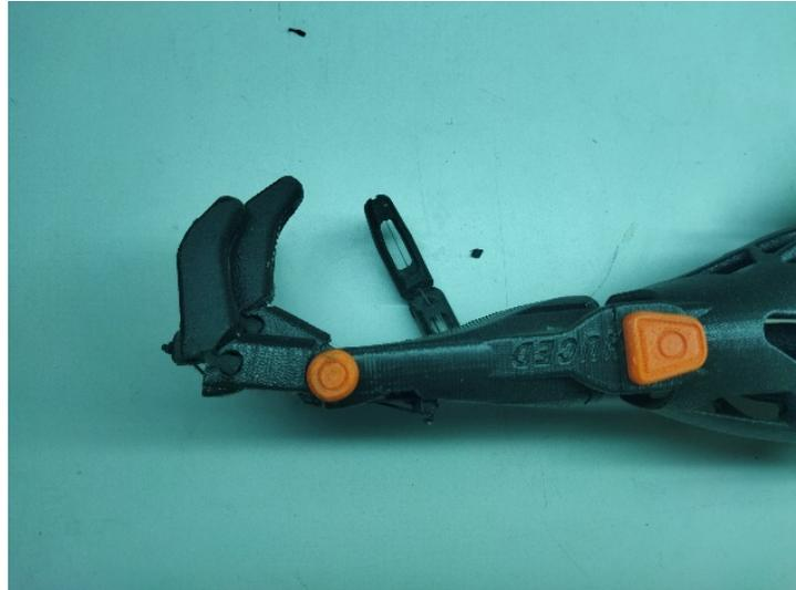
**Figure 2:** Image of the arm robot with a focus on its finger prosthetic arms.
