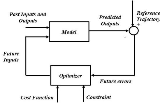
Figure 1: MPC Structure.
