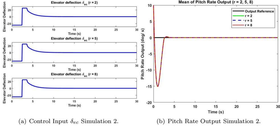
**Figure 4:** Control Input & Pitch Rate Output for Different Polynomial Orders ( $r = 2, 5, 8$ ).
