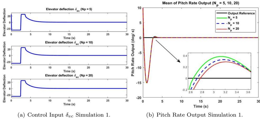
**Figure 3:** Control Input & Pitch Rate Output for Different Prediction Horizon ( $N_p = 5, 10, 20$ ).
