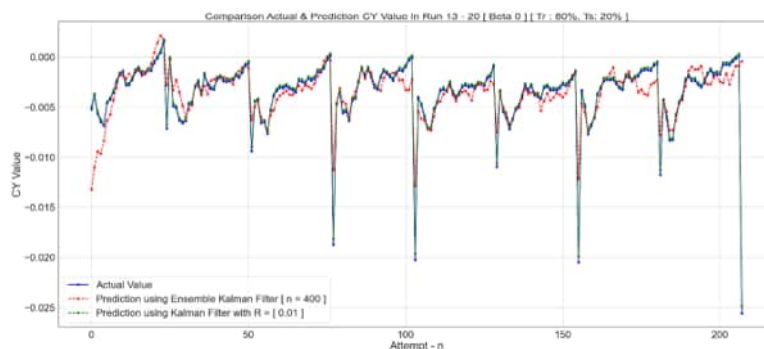
Figure 2: CY Value Prediction Plot using the EnKF method of 400 ensembles with observation models of 0.8 and KF.
