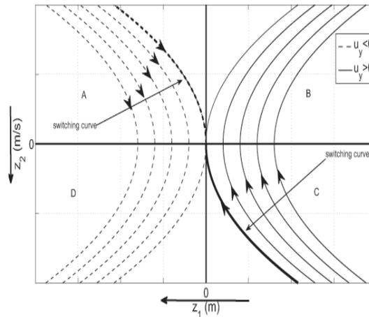
**Figure 5.1:** Qualitative shape of the curves on the phase plane of the double integrator subsystem ( $z_1$  vs.  $z_2$ ) in case of constant thrust along the  $y$  axis for both the Hill–Clohessy–Wiltshire and the Schweighart–Sedwick models.
