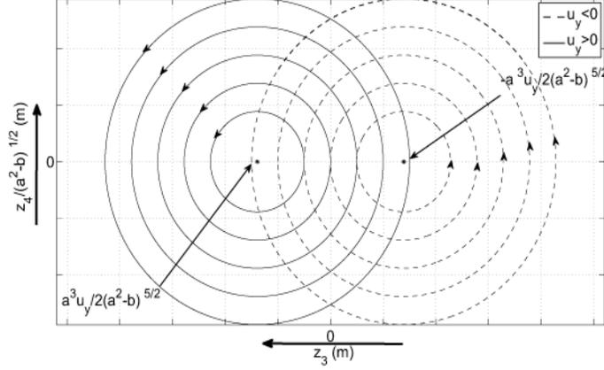
**Figure 5.2:** Qualitative shape of the curves on the phase plane of the harmonic oscillator subsystem ( $z_3$  vs.  $z_4$ ) in case of constant thrust along the  $y$  axis for both the Hill–Clohessy–Wiltshire and the Schweighart–Sedwick models.
