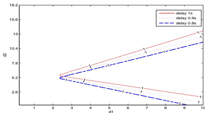
**Figure 6.** Deterministic stability for three different delays  $\tau = 1$ ,  $\tau = 0.9$ ,  $\tau = 0.8$ . The intersecting region of these triangular boundaries is stability region in deterministic sense.
