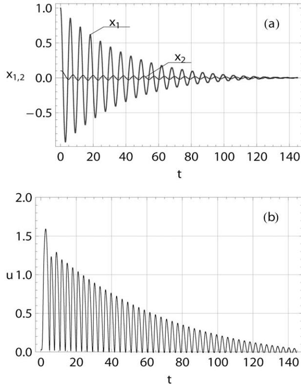
**Figure 3:** Beat suppression under the reduced time increment  $h = 0.001$  and the same weight parameter  $\lambda = 1.0$ : (a) the system response, (b) control input - the damping ratio of second oscillator.
