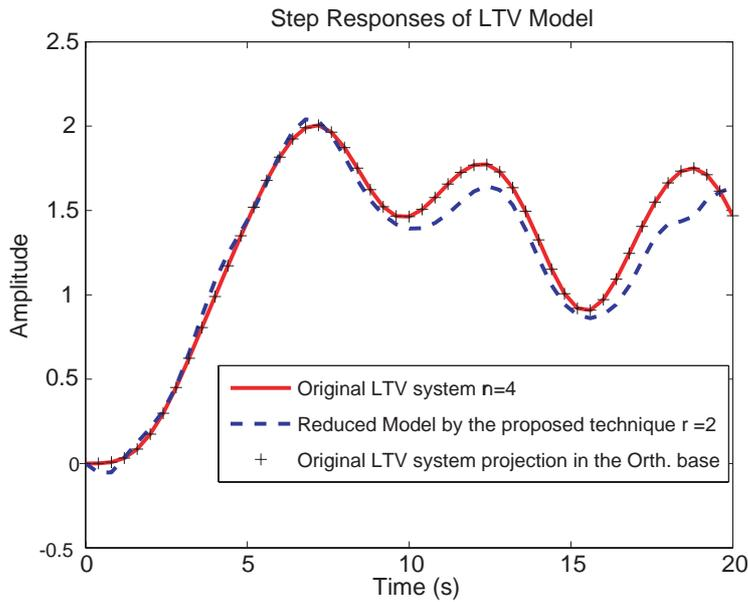
**Figure 4:** Step responses of the original LTV system, the projected system into Legendre shifted polynomials and the reduced order LTV model.
