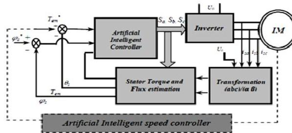
Figure 2: Schematic diagram of DTC-PMSM control.
