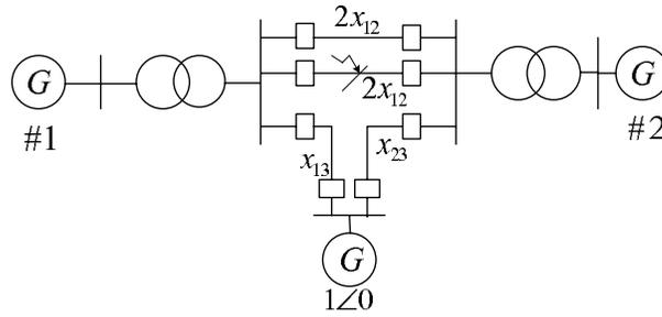
Figure 7.1: The two machine infinite bus test system.
